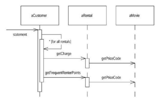
Figure 1.9. Sequence diagram before extraction of the totals
